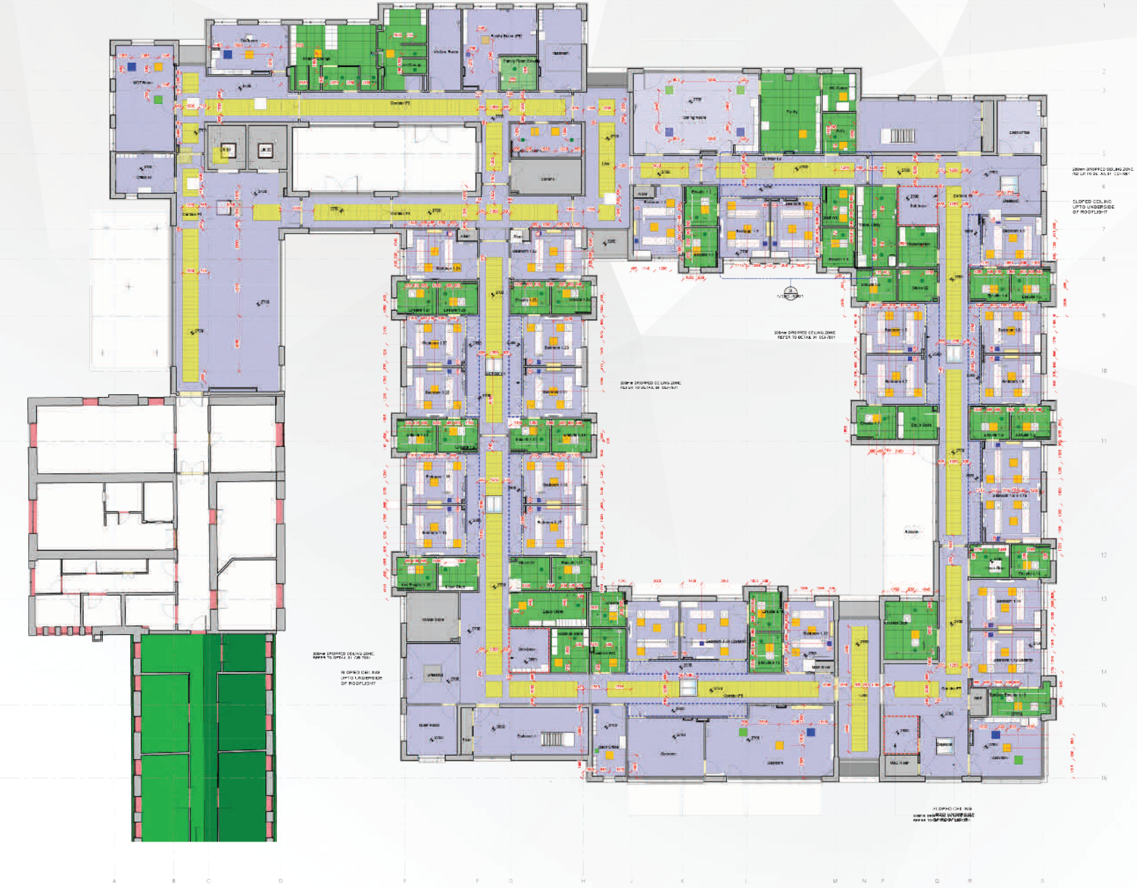
FIRST FLOOR REFLECTIVE CEILING PLAN
